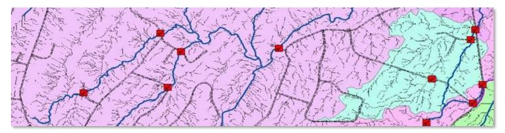
GroundPoint developed an enhanced surface model from the original LiDAR data and edited it iteratively to reflect actual field conditions. The process identified improvements in the culvert inventory point data such as missing culverts, culvert location adjustments, and flagging potentially erroneous entries. The culvert inventory data was based on a standard data model provided by the North Atlantic Aquatic Connectivity Collaborative (<u>http://streamcontinuity.org</u>). The improved culvert
