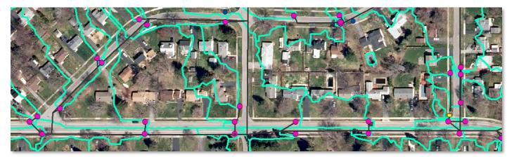
GroundPoint initially developed an enhanced surface model from the County LiDAR data. The process included some limited editing of the surface model associated with culverts, and critically evaluating the point cloud in areas of concern to ensure flow was not impacted by digital artifacts. In most cases, the LiDAR data provided excellent coverage of the surface. An unexpected value of the project was an independent QC of the Town's Storm Water GIS data, which helped
